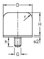
$$\begin{array}{lll} D & = 63 \\ G & = M10 \\ H & = 50 \\ h & = 28 \\ Load capacity F (kN) = 37.5 \\ Load capacity f (mm) = 28 \\ Load capacity W (J) & = 280 \\ r & = 12.5 \\ \end{array}$$
